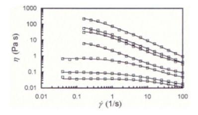
Figure 2. Experimental flow curves (20°C; 0.1M NaCl) for cactus mucilage solutions at concentrations (% w/w)(from top) of: 5.8, 3.10, 2.9, 1.6, 0.8, 0.5 and 0.4.
