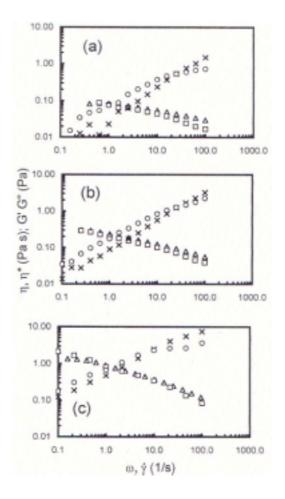
Figure 1. Dependence of storage, G'( $\Delta$ ), loss, G''(o) mechanical moduli, and dynamic viscosity,  $\eta^*$  ( $\Box$ ), on frequency,  $\omega$ , (strain 0.05) and of steady-shear viscosity,  $\eta(\diamond)$ , on shear rate,  $\gamma$ , for cactus mucilage solutions at concentrations (% w/w; 20°C in 0.1M NaCl) of: a) 1.0; b) 1.6; and c) 2.0.
