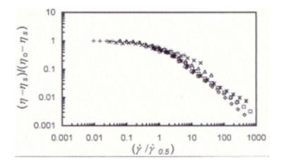
Figure 3. Generalized shear-thinning curves (20°C) obtained from the experimental flow curves in Figure 2 by scaling measured values of 0 to the maximum "zero-shear" viscosity ( $\eta$ ) for each solution, and similarly scaling  $\gamma$  to the shear-rate required to reduce  $\eta$  to  $\eta_0$  /2. Mucilage solutions concentrations (% w/w in 0.1M NaCl) were: 5.8 ( $\Diamond$ ), 3.10( $\Box$ ), 2.9(o), 1.6(\*), 0.8( $\Delta$ ), 0.5(x), 0.4(+).
